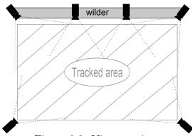
This schema gives an idea about how the VICON system is tracking 3D motion. It covers almost the entire area in front of the wall with enough precision and a high enough refreshing rate to provide good interaction (respectively up to 0.5mm and 250 fps). As we have seen before, mid-air gesture is an option for distant interaction.
