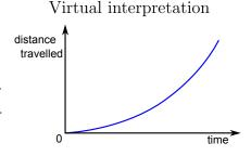
The **First order area** technique uses a zero order pan movement inside a given area and first order pan movement beyond. It is inspired by RubberEdge, presented by Casiez et al. [5], and tries to extend user reach on a wall. This technique was interesting because it was extending user reach, meaning that when the user had his arm almost straight, he could still interact by switching to first order of control and avoid clutching.
